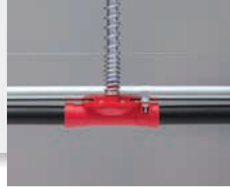
Slope Neutralizer Reduces slope pressure by a preset amount, requires no adjustment and maintains system pressure setting even when birds are not drinking. Required in sloped houses only.
