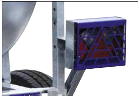
Lights protected by metal grills
