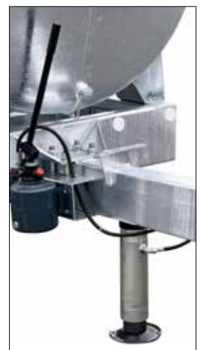
Hydraulic stand with pump and reserve supplied as standard for the 8000 L model. Assembly equipped with a 1/4 turn valve and push-pull sockets from which the hose can be removed when the bowser remains in the field.
