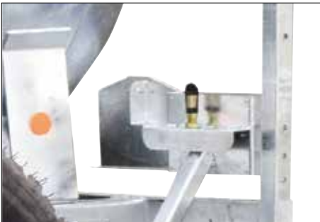
Protected wiring. Rear flashing light socket.
