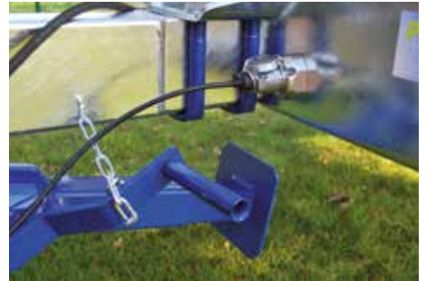
Electrical extension from the frame to the tractor (provided), preventing damage to the wiring harness by animals. Rear lights connected by passing the wire directly into the frame.
