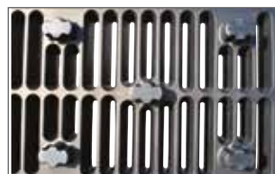
8 staggered feet beneath slatted floor avoid blockage by long fibres during cleaning.
